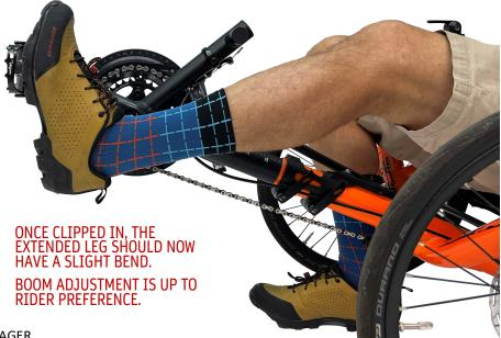
CLOSE BOOM CLAMP BY TIGHTENING THE QUICK RELEASE NUTS ON BOTH HANDLE. THE BOOM SHOULDN'T ROTATE WHILE EDALING.
