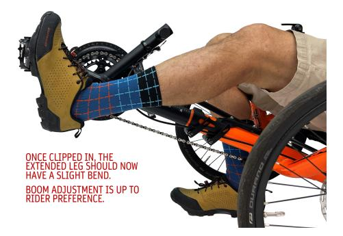
CLOSE BOOM CLAMP BY TIGHTENING HE QUICK RELEASE NUTS ON BOTH HANDLE. THE BOOM SHOULDN'T ROTATE WHILE EDALING.
