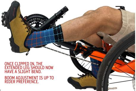
CLOSE BOOM CLAMP BY TIGHTENING THE QUICK RELEASE NUTS ON BOTH HANDLE. THE BOOM SHOULDN'T ROTATE WHILE PEDALING.
