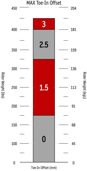
IF THE RIDER CAN NOT SIT ON THE TRIKE WHEN PERFORMING THE TOE ADJUSTMENT THEN FOLLOW THE STEPS TO APPROXIMATE THE CORRECT TOE FOR THE RIDERS WEIGHT:
