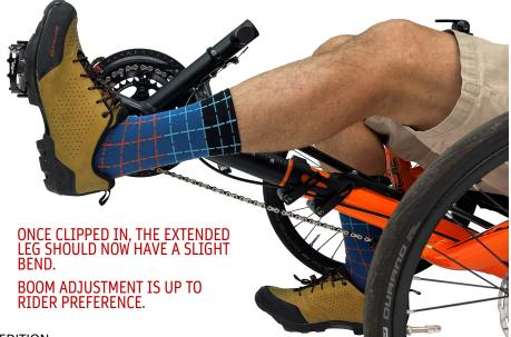
CLOSE BOOM CLAMP BY TIGHTENING HE QUICK RELEASE NUTS ON BOTH HANDLE. THE BOOM SHOULDN'T ROTATE WHILE PEDALING.
