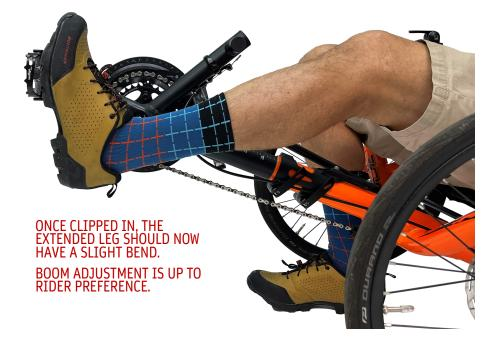
CLOSE BOOM CLAMP BY TIGHTENING HE QUICK RELEASE NUTS ON BOTH HANDLE. THE BOOM SHOULDN'T ROTATE WHILE EDALING.
